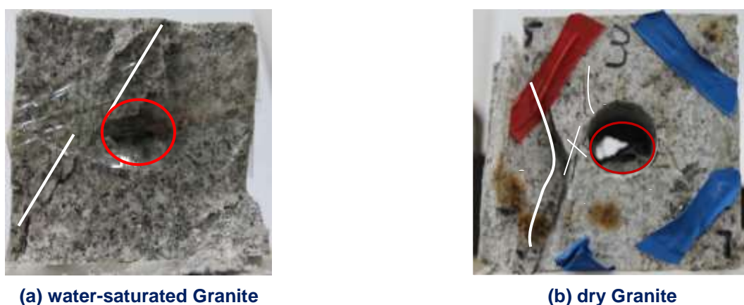
Fig. 6. The fissure damage morphology of dry and saturated Granite sample.
