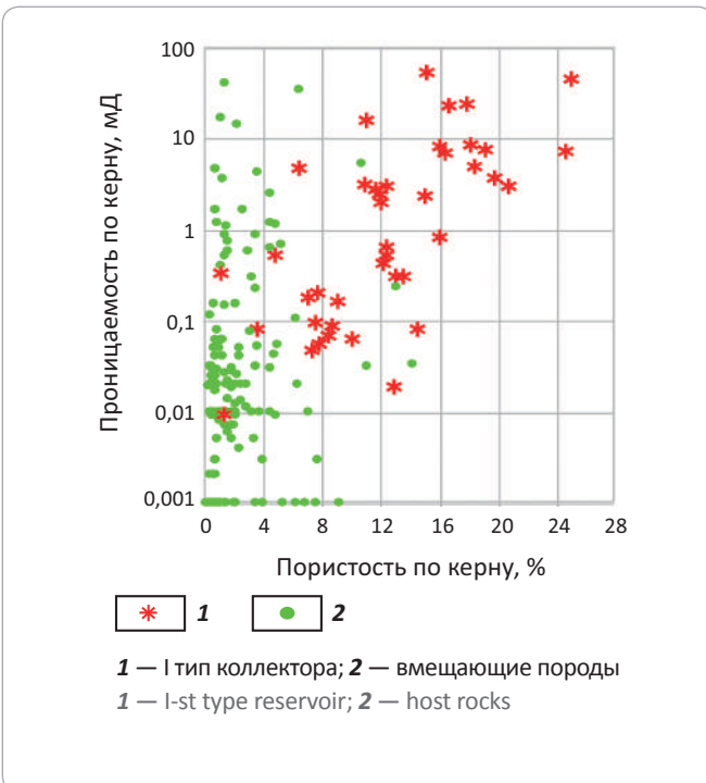
Fig. 5. Porosity vs permeability crossplot for I-st type reservoirs and the rest of the section (wells 1, 2, 3, 4, 6)
