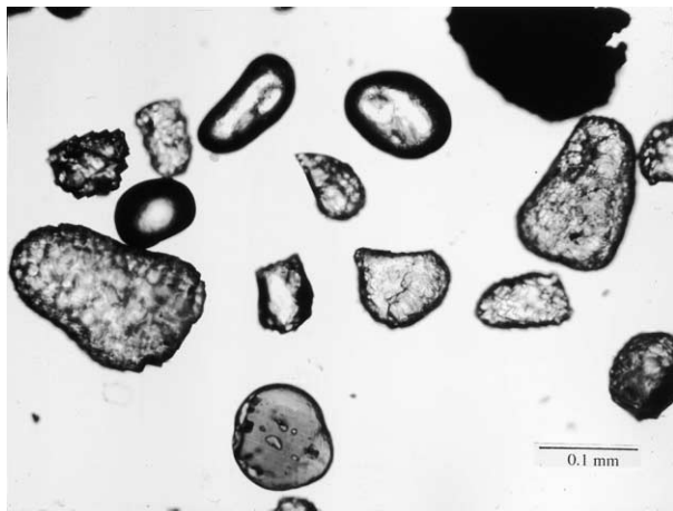
Figure 2. Photomicrograph of well-rounded accessory minerals from the St. Peter Sandstone, Wisconsin (zircon, tourmaline, garnet, ilmenite; grain mount in plane-polarized light).
