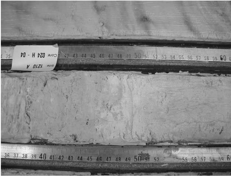
Figure 12.6. Cretaceous–Tertiary boundary at a depth of 219.82 m below the seafloor at site 1210A of Ocean Drilling Project Leg 198 (Shatsky Rise, Pacific Ocean). All sediments are calcareous abyssal plain deposits. Lowermost Tertiary (Danian) toward the left is separated by several centimeters of bioturbated sediment from underlying uppermost Cretaceous (Maastrichtian) deposits. The bioturbated zone contains micro- and nanofossils both older and younger than the boundary plus \sim 0.05 -mm microspherules distributed around the earth from the Chicxulub impact site (see text). (Photo courtesy of Harumasa Kano.)
