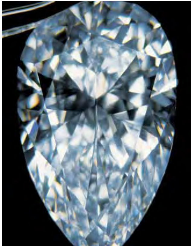
Figure 15. Occasionally graining is observed that exhibits an overall rain-like appearance and is noticeable face up through a range of motion. While such graining does not diminish transparency, as seen in this 10+ ct diamond (left), its obvious visual disruption to the appearance of the diamond (above) results in a report comment noting “Transparent internal graining is present.” Photos by Vincent Cracco; photomicrograph magnified 30x.
