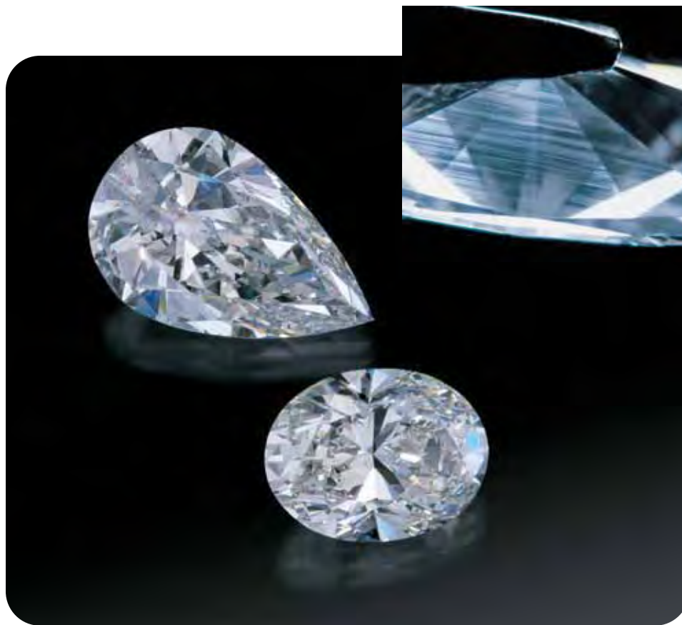
Figure 1. The 30+ ct pear shape and 18 ct oval shown here are representative of the large colorless to near-colorless diamonds in which whitish graining may affect the clarity. This effect is often misunderstood due to the elusive nature of such graining. The photomicrograph illustrates a classic example of the cottony banding encountered in whitish graining that will have an impact on the clarity grade. Photo © Harold & Erica Van Pelt; photomicrograph by Vincent Cracco, magnified 21×.
