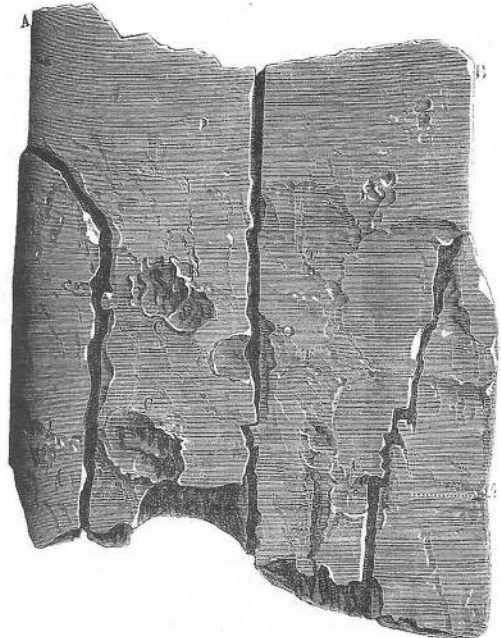
Fig. 12. Detail of portion of steel bar, broken and eroded by dynamite explosion (Daubrée 1879c, fig. 234, p. 651).
