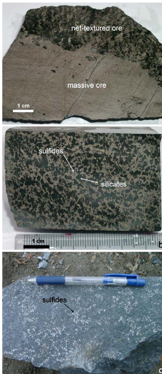
Fig. 2 Three ore types of the Baimazhai deposit. (a) Sharp boundary of massive ore and net-textured ore; (b) polished drill core sample of net-textured ore; (c) disseminated ore
