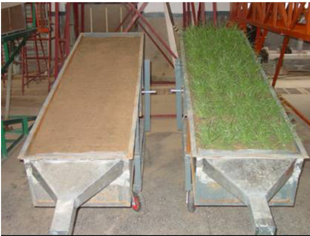
Figure 1 Contrast of a bare soil plot and a grassplot before simulated rainfall.
