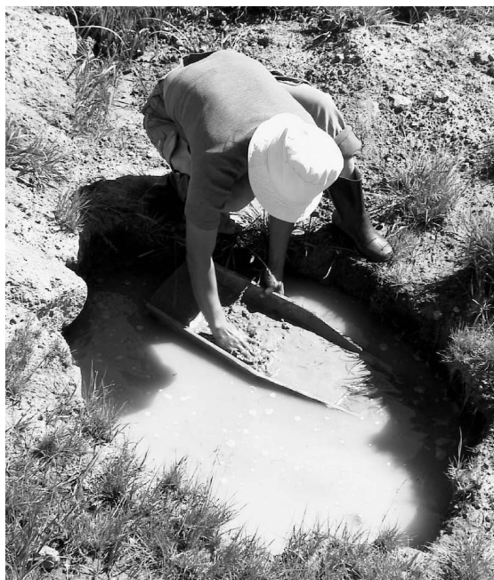
FIG. 7. Concentration of heavy minerals near the Shavryn Tsaram gemstone deposit using a wooden Mongolian-style pan.
