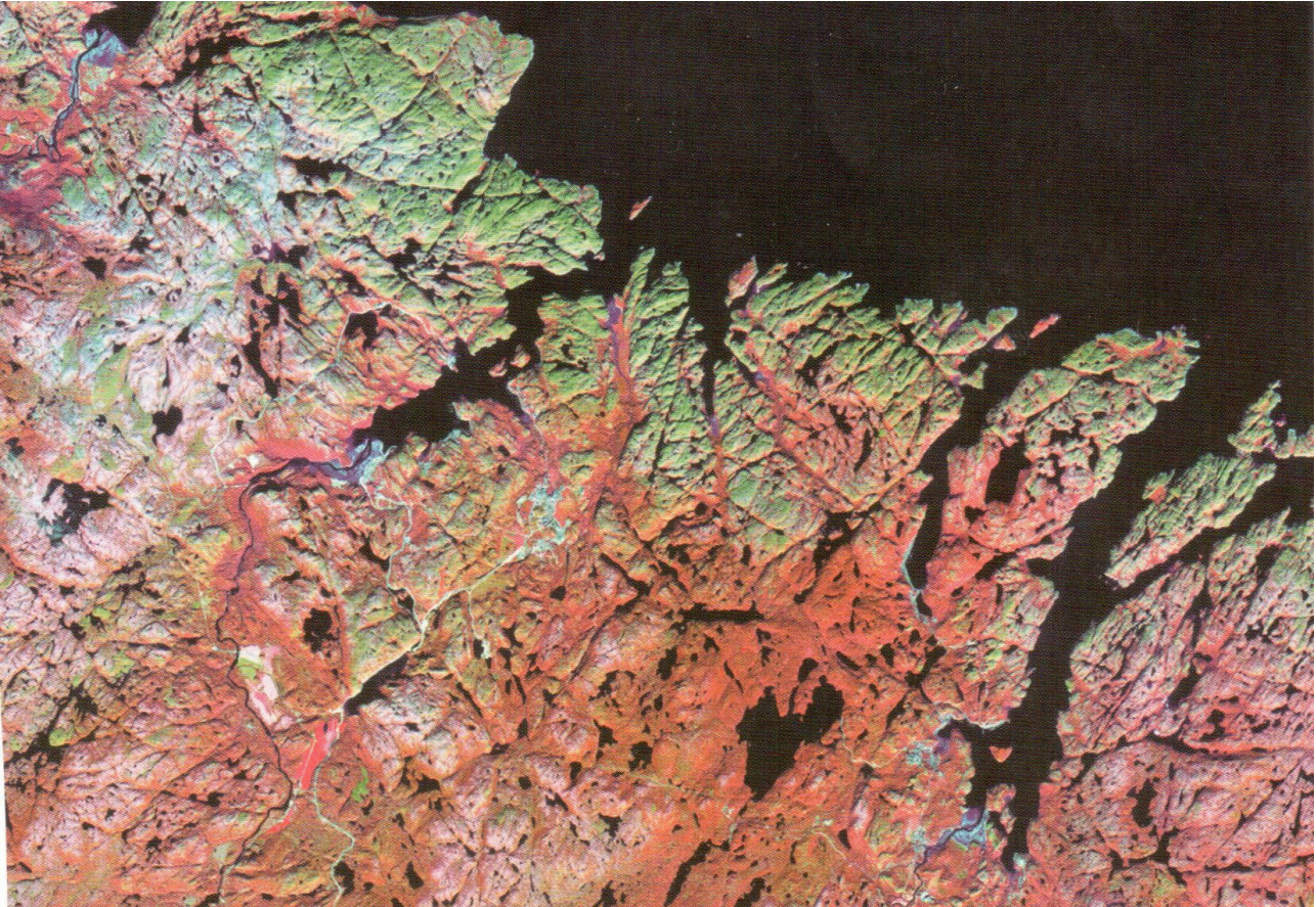
Fig. 2. A space image of the north-eastern part of the Kola Peninsula: the Murmansk geoblock of Archean granitoids divided by a dense network of neotectonic fractures and fissures. The intersecting fractures and fissures form numerous lakes, which are the deepest at the sites of fracture intersection. The coast of the Barents Sea is complicated with fracture-tectonic zones, fjords
