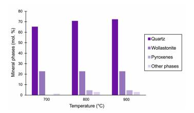
**Fig. 2.** Charoite rock decomposition products (mol %) using thermodynamic modeling by "Selector" PC.
