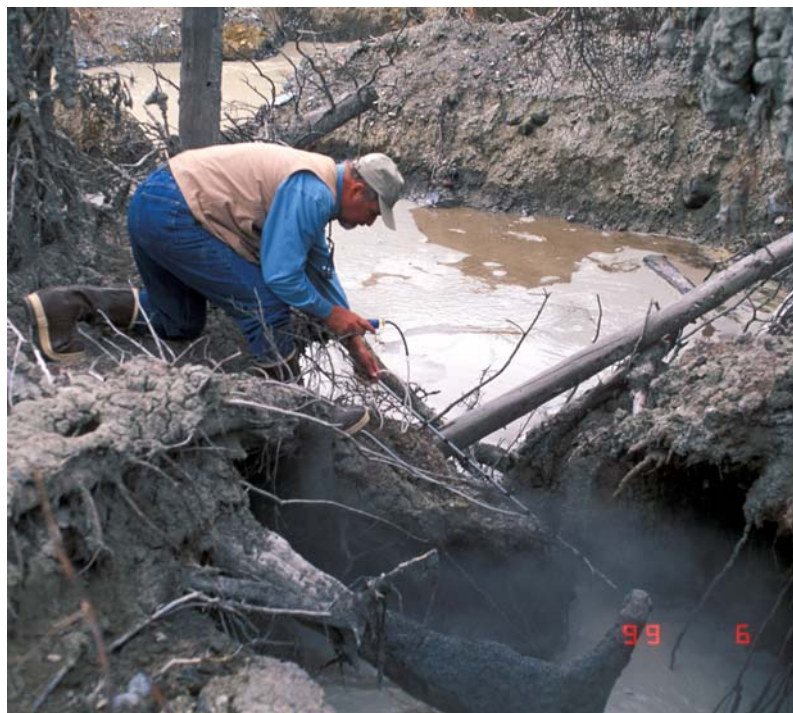
Figure 7. Mike Sorey (USGS) measures CO 2 flux in Pit 3, Main vent area (fig. 5). Photo by R.G. McGimsey, June 22, 1999.
