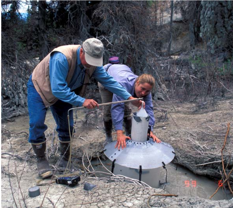
Figure 6. Mike Sorey (USGS) and Cindy Werner (Penn State University) measure CO 2 flux at Pit 6 of the Main Vent area (fig. 5). Photo by R.G. McGimsey, June 22, 1999.
