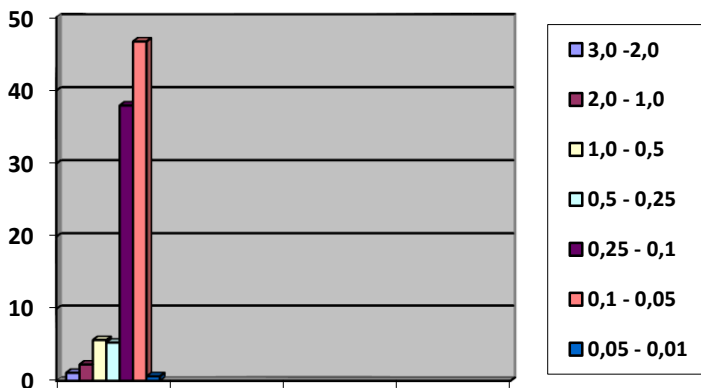
Fig. 6. Histogram of granulometric composition of the Novopetrivska suite and sands in the outcrop
