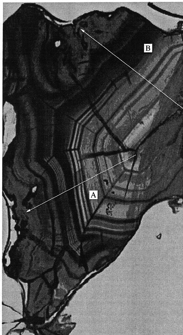
Fig. 1. Photo of the surface of the agate specimen from the Pavlodar region, Kazakhstan. The profile A is 18 mm long and the profile B is 17.1 mm long.
