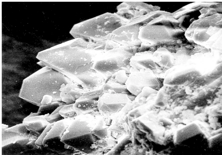
Fig. 1. SEM image of the aggregates of bradaczekite crystals. Magnification: ~ 600×.
