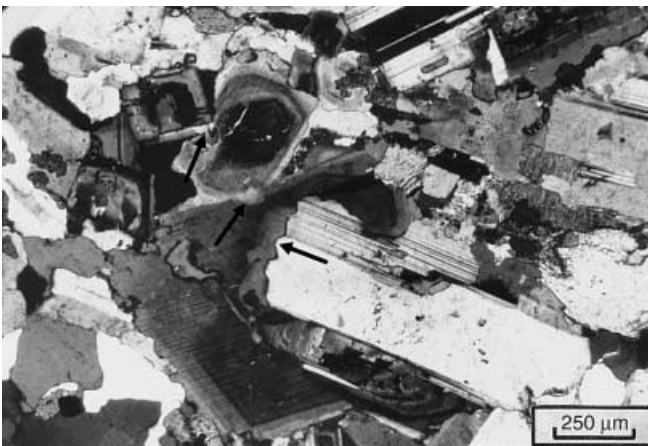
Fig. 9 Micrograph (crossed polarizers) of a tonalite from the Adamello Pluton (Southern Alps, Italy). Note the indentations (arrows) of plagioclase grains into each other, cross-cutting the euhedral zonation rims. Indentations are inferred to result from dissolution at grain-to-grain contacts in the presence of melt
