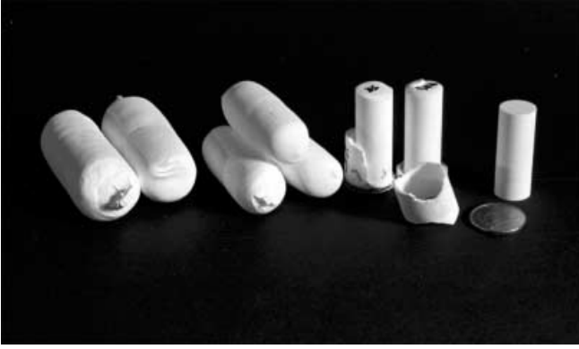
Fig. 4 Photographs of products obtained at various stages during fabrication. From left to right CIPed greenbodies, fired material and machined samples (10 mm in diameter by 25 mm in length)
