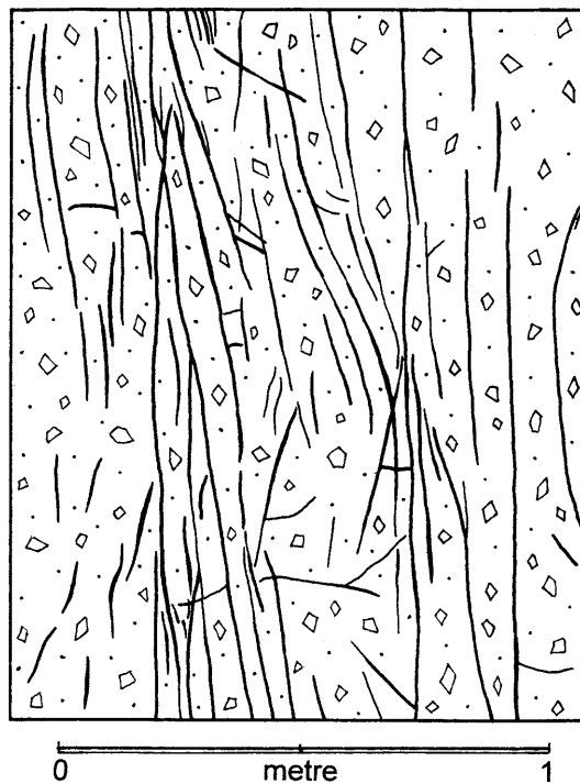
Fig. 2 Typical sheeted vein zone cutting diatreme breccia in the Cripple Creek gold deposit, Colorado, United States (extracted from a drawing of the Captain vein in the Portland mine by Lindgren and Ransome 1906). Individual seams are vuggy and lined with crystalline aggregates of quartz, fluorite, dolomite, pyrite, calaverite and minor amounts of other minerals. Note the marked contrast with normal low-sulphidation epithermal quartz veins
