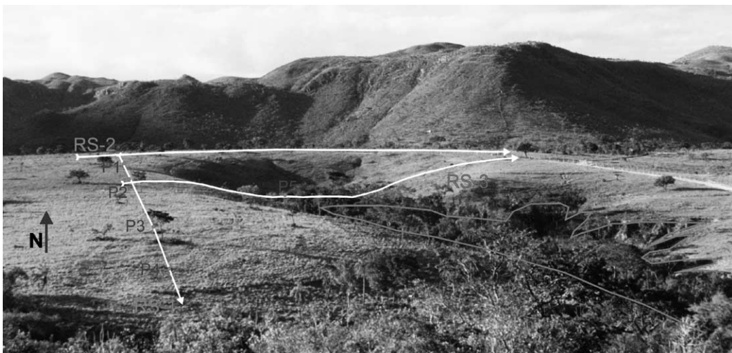
Fig. 2. View of the hollow, the survey lines, the position of the weathered profiles: borehole (P 1–5), and the contour of the gully (right side).
