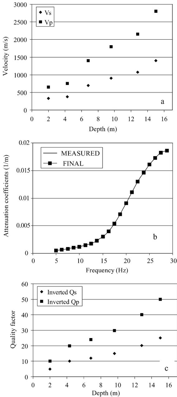
Fig. 6. A synthetic example. (a) P-wave and S-wave velocities of a six-layer model. (b) Input data: assumed known attenuation coefficients labeled “Measured” and calculated attenuation coefficients labeled “Final” based on inverted quality factors in (c).
