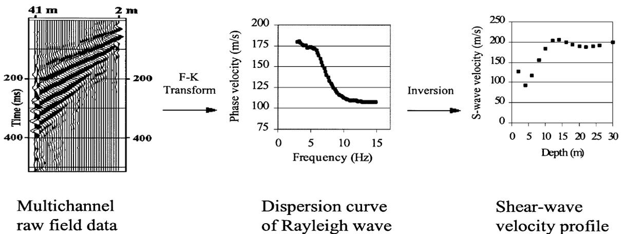
Fig. 2. A diagram of the MASW method. Multichannel raw field data, which contain enhanced Rayleigh wave signals, are acquired. Rayleigh wave phase velocities are extracted from the field data through a direct wavefield transformation method by Park et al. (1998). The phase velocity, finally, is inverted for a shear-wave velocity profile ( $V_s$  vs. depth).
