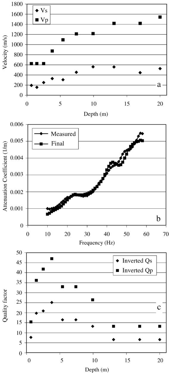
Fig. 8. Inversion results from data in Fig. 7. (a) Inverted S-wave velocities of a 10-layer model by using the MASW method with P-wave velocities determined based on the first arrivals of the input data. (b) Attenuation coefficients labeled “Measured” were calculated by Eq. (6) and those labeled “Final” were calculated based on the inverted quality factor model (c).
