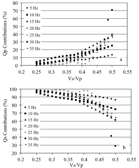
Fig. 4.  $Q_P$  contributions to Raleigh wave attenuation coefficients (a) and  $Q_S$  contributions to Raleigh wave attenuation coefficients (b).  $Q_P$  contributions become significant when  $V_S/V_P$  is about 0.5.
