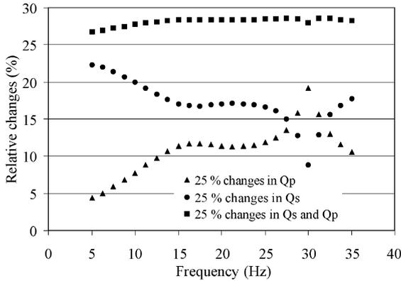
Fig. 5. Sensitivity of Rayleigh wave attenuation coefficients to  $Q_P$  and  $Q_S$  with  $V_S/V_P$  being equal to 0.5.
