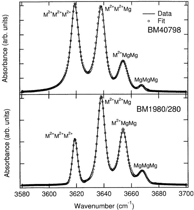
**Fig. 6** Two typical infrared absorption spectra from each sample showing fine structure in the hydroxyl-stretching region. *Background* has been removed and *peaks* fitted on the basis of the minimum number required and the lowest residual between observed and fitted spectra
