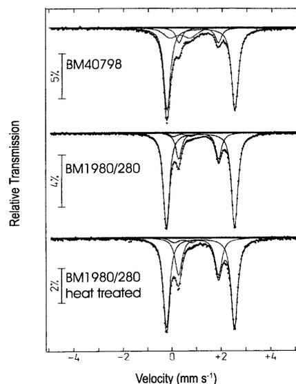
Fig. 5 Mössbauer spectra of the two samples showing quadrupole doublets of  $^{57}Fe$ , resolved into contributions from  $Fe^{2+}$  at M(1,2,3) = outer doublet,  $Fe^{2+}$  at M(4) = inner doublet and  $Fe^{3+}$  = broad doublet with low intensity. Note that two separate samples of BM1980/280 were analyzed, one of which had been to high temperature at ISIS
