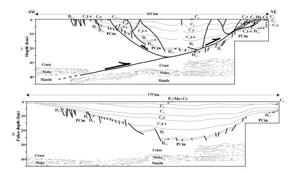
Figure 4. A: Supplemented depth section along DOBREflection-2000 and southernmost part of profile extension of 2001. B: Palinspastic reconstruction along depth section prior to shortening.
