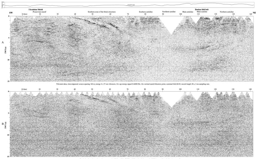
Explosive data, time-migrated: source spacing 2940 m; 80 kg TNT in 10-30 m shot holes; nominal fold 4; record length 64 s; 4 ms sampling rate.
