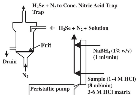
Fig. 1. Schematic diagram of the new Continuous Flow Hydride Generation System developed for purification of Se before TIMS analysis. The frit is a fine-glass frit (4–5.5  $\mu\text{m}$ ).
