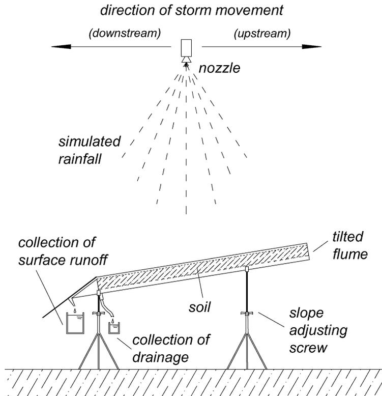
Fig. 1. Schematic representation (side view) of the soil flume and hydrological variables involved in the laboratory experiments.
