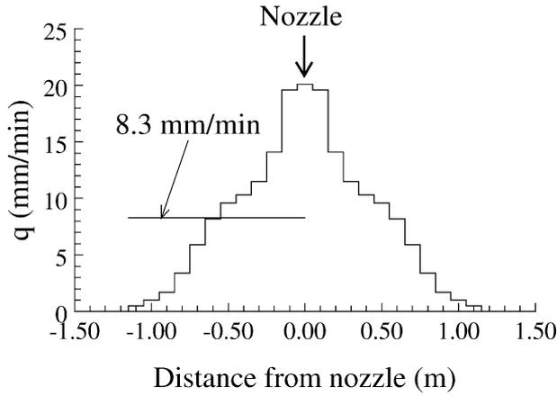
Fig. 3. Distribution of rainfall intensities supplied by the nozzle (static) on a horizontal surface, for an operating pressure of 0.5 bar, at a height of 1.5 m.
