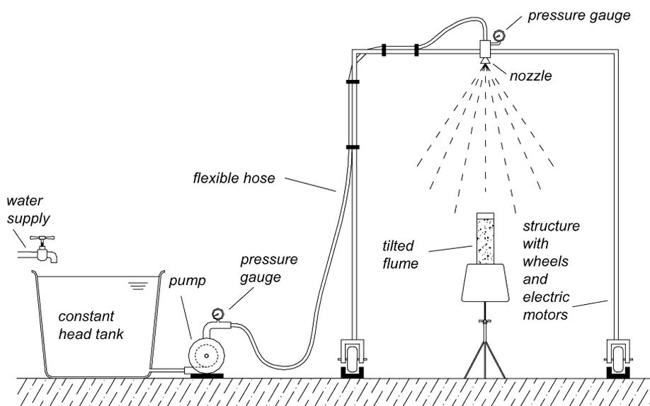
Fig. 2. Schematic representation (front view) of the rainfall simulator including the connections with the water supply and the movable support structure.
