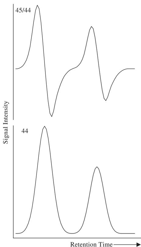
Fig. 1. A characteristic GC-IRMS trace. The lower chromatogram shows the mass 44 signal, which is analogous to a gas chromatogram. The upper trace shows the 45:44 mass ratio which reflects the isotopic composition of  $\text{CO}_2$  entering the mass spectrometer source. Note the characteristic 'swings' in the 45:44 ratio trace which reflects the fact that compounds containing greater quantities of  $^{13}\text{C}$  elute earlier.
