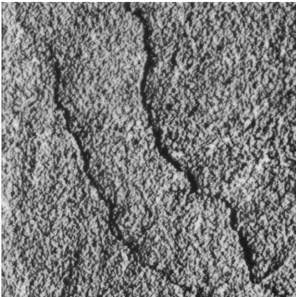
Fig. 10. Deflection image of retreating steps on the (001) surface of apophyllite at 130\text{ }^{\circ}\text{C} ( \text{pH} = 5.6 , P = 10\text{ bar} ; steps are stepping down from left to right). The morphology of the steps is rough, their height is about a few nanometers. Scan field 6 \times 6\text{ }\mu\text{m}^2 .
