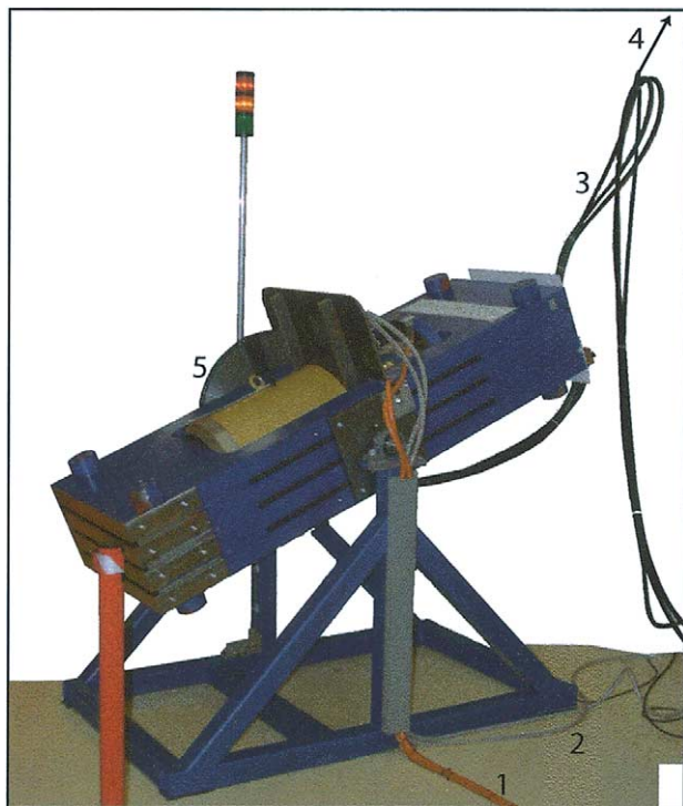
Fig. 2. Rocking multianvil device; 600-ton O-frame press with 6/8 cylindrical multianvil module. 1: Power cables; 2: cooling water hoses; 3: hydraulic pressure hoses; 4: pull-out wire; arrow indicates where fixed to the wall; 5: sprocket wheel.
