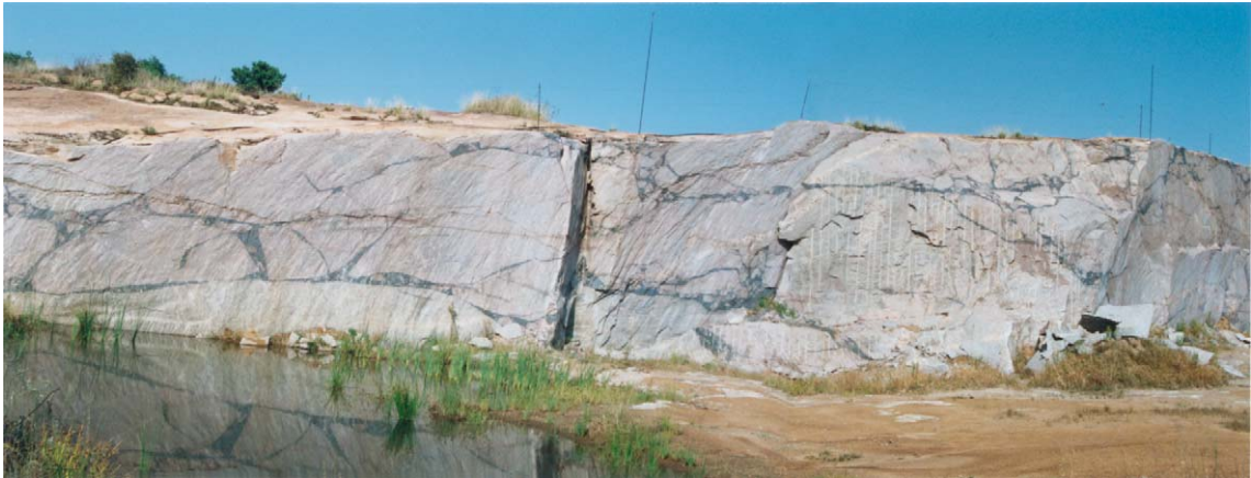
Fig. 21. Pseudotachylite zone in Esperanza Quarry, Wittekoppies 169 Farm (western Vredefort Dome; latitude 27^{\circ}06'26''\text{S} ; longitude 027^{\circ}18'52''\text{E} ). On the upper, horizontal level of the quarry, the zone is straight and dike-like with branches towards the quarry wall. The dike trends more or less parallel to the quarry wall.
