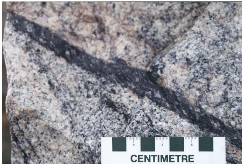
Fig. 25. Kinematic indicators in pseudotachylite veins suggestive of sinistral shear. Dimension stone block at Esperanza Quarry (Wittekopies 169 Farm, western Vredefort Dome; latitude 27°06'26"S; longitude 027°8'52"E).
