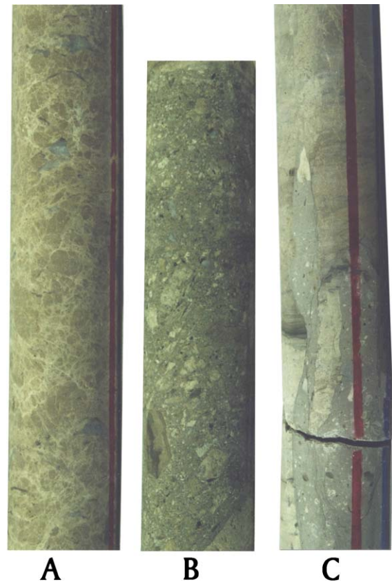
Fig. 28. Clastic-matrix breccias, Chicxulub Structure, Yaxcopoil 1 drill hole, Yucatan, Mexico. (A) Monomict breccia in dolomite (1318.95 m). (B) Polymict breccia vein (all of core section shown; 1341.75 m). (C) Polymict breccia vein (1316.0 m).
