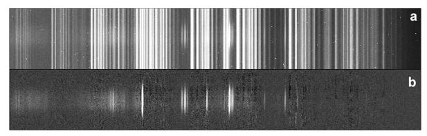
Fig. 1. Raw CCD part frame of the ESO VLT meteor of May 12, 2002: a) meteor + sky; b) meteor after sky subtraction.
