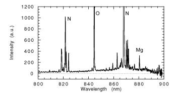
Fig. 3. Perseid meteor spectrum obtained with a slit-less CCD spectrograph on August 13, 2002 at 10:24:33 UT. Note the presence of the meteoric metal Mg I emission line not seen in the ESO VLT spectrum.
