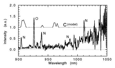
Fig. 6. The newly opened wavelength range from 900 to 1050 nm, with the superimposed air plasma model (dashed line). A similar model for LTE C I line emission at 4,340 K is displaced upward by 1 unit to facilitate comparison. The rise of the spectrum toward long wavelengths is possibly an artifact of the reduction process because the signal is weak and the instrument response is falling off.
