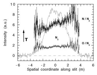
Fig. 5. Ratio of N/N<sub>2</sub> and O/N<sub>2</sub> intensities along the length of the slit from top (negative) to bottom (positive). The nitrogen band intensity profile is shown for comparison. The line ratios increase with temperature when a higher fraction of N<sub>2</sub> is dissociated.
