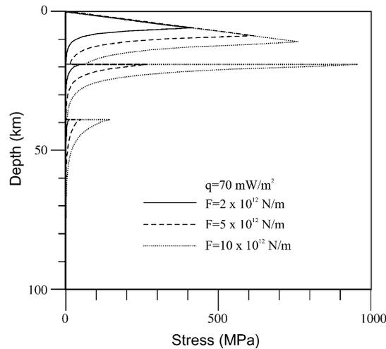
Fig. 7. Stresses developed in a V-type model in WLF at different applied forces and surface heat flow  $q=70 \text{ mW m}^{-2}$ . The dashed line ( $F=5 \times 10^{12} \text{ N m}^{-1}$ ) is the same as in Fig. 3d.
