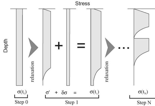
Fig. 2. Schematic illustration of the “viscous” (V-type) model. Step 0: initial (elastic) stress  $\sigma(t_0)$  arising from a constant force boundary condition. Step 1: initial stress after relaxation  $\sigma'$ , according to Eq. (4); stress  $\delta\sigma$  added to  $\sigma'$  (giving  $\sigma(t_1)$ ), compensating the implicit force reduction due to the relaxation (i.e. difference between  $\sigma(t_0)$  and  $\sigma'$ ) in order to maintain the constant force boundary condition.
