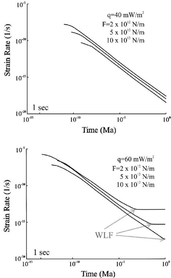
Fig. 4. Evolution of strain rate through time in the V-type model for two different heat flow values and various applied forces (higher force, higher strain rate). The lithosphere reaches a critical stress regime when the strain rate becomes constant in time (labelled WLF—whole lithospheric failure).
