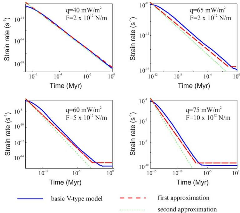
Fig. A.2. Strain rate vs. time dependencies in the V-type model, with approximations as discussed in the text for different applied forces and surface heat flows.
