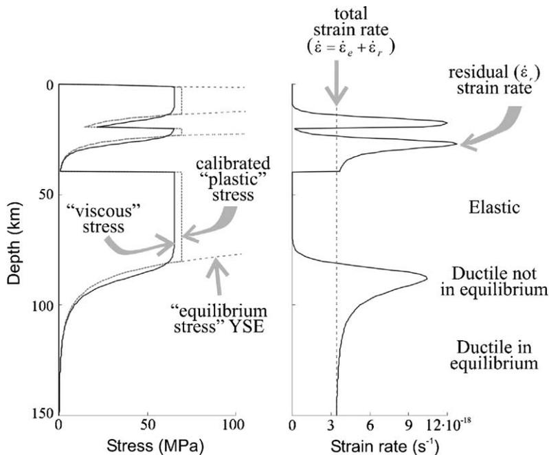
Fig. 8. Comparison of stresses for the calibrated P-type model and stresses for the V-type model (left) and the strain rate distribution with depth in the V-type model with  $F=5 \times 10^{12} \text{ N m}^{-1}$  and surface heat flow  $q=45 \text{ mW m}^{-2}$  after 1 Myr.
