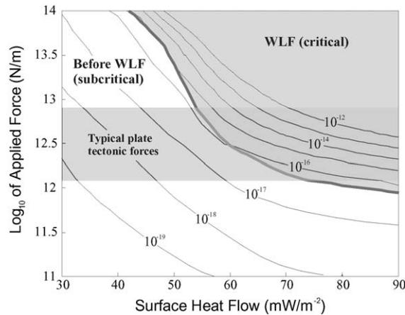
Fig. 5. Calculated strain rates in the V-type model after 1 Myr of loading as a function of applied force and heat flow; the shaded region is where the stress state has become critical by this time, where WLF can be considered to have occurred. The horizontal shaded band indicates the range of typical plate tectonic forces in the lithosphere (e.g. Turcotte and Schubert, 1982).
