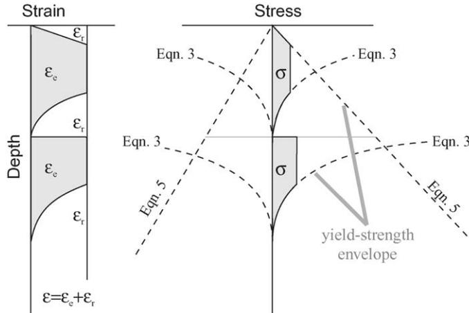
Fig. 1. Schematic illustration of the “plastic” (P-type) model. Strain with depth is shown at the left; it comprises an elastic component  $\epsilon_e$  (shaded part) and a non-elastic (residual) component ( $\epsilon_r$ ), the sum of which (total strain) is constant with depth. The elastic strain is defined by the stress, which does not exceed  $\sigma_{\text{yield}}$  as defined by Eqs. (5) and (6).
