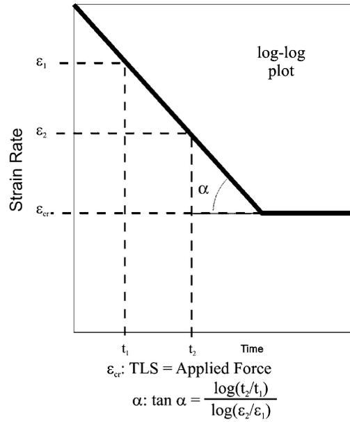
Fig. A.1. Simplified strain-rate vs. time dependence in the V-type model.
