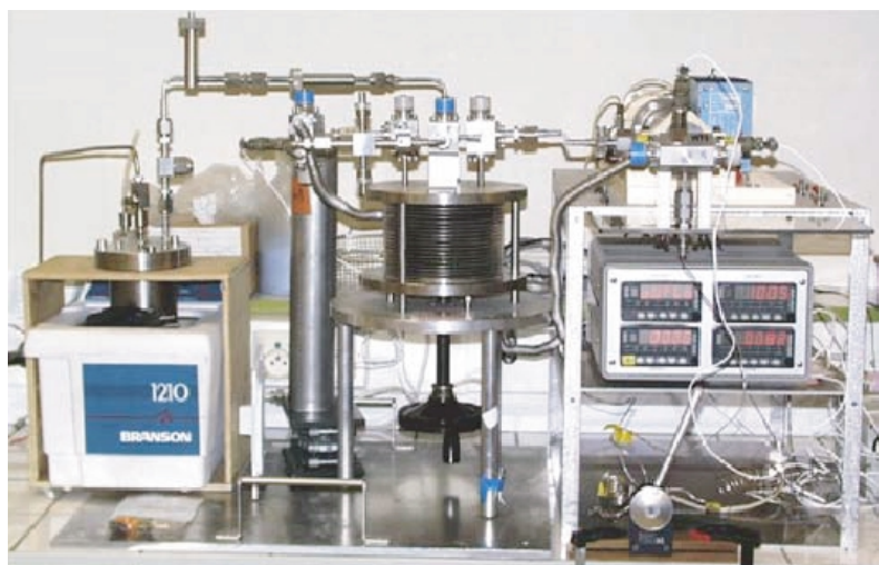
Fig. 2. Schematic diagram and photograph of the gas extraction line.
