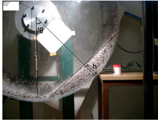
Figure 2. The rotating drum used to measure \mu_d , \mu_c and \tau_0 . \theta is defined as shown.
