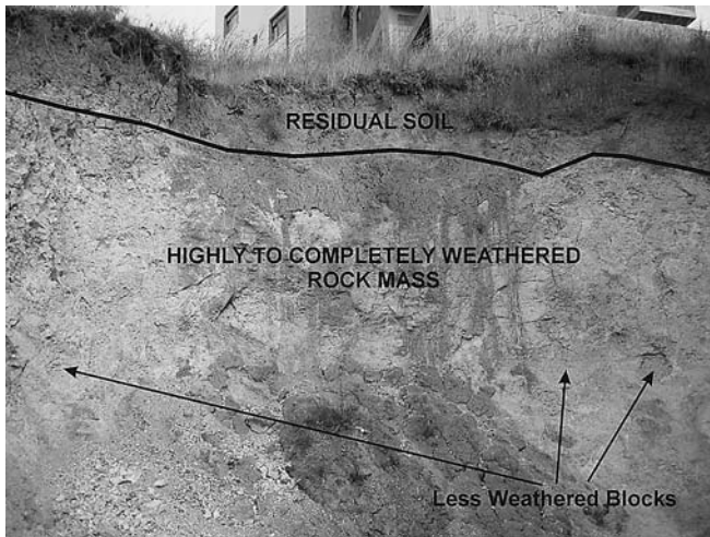
Fig. 4 Photograph of the weathering profile in the andesite of the Pursaklar region
