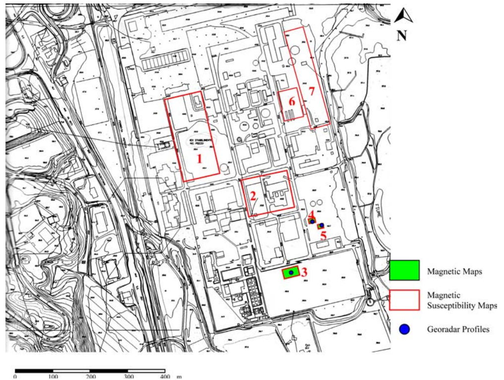
Fig. 4 Map of Ferrandina industrial settlement with the location of the magnetic susceptibility, magnetometric, and GPR surveys
