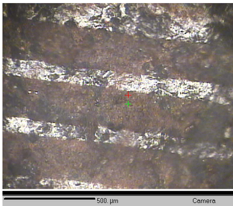
Fig. 4. Photomicrograph of a rock varnish surface (SJ-CT1) following a single laser ablation pass (250 \mu\text{m} beam). The dark, lustrous areas between raster traces are representative of typical varnish-bearing surfaces before laser ablation.
