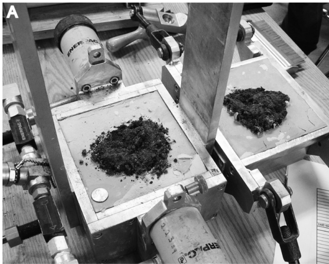
Fig. 4. Laboratory direct shear tests. (A) Sample of PM-002 in direct shear apparatus after shear testing. Penny for scale. (B) Mohr–Coulomb strength envelopes for fracture surfaces in PM-001 and PM-002.
