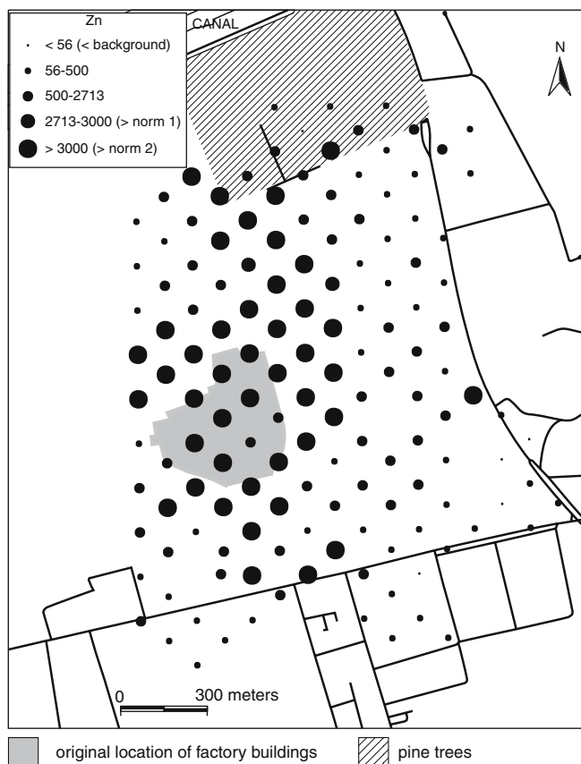
Fig. 2 Distribution pattern of Zn on the site. Background, norm 1 and norm 2 refer to the background and reference values according to the Vlarebo (Anonymous 1996) (see Elemental analysis of polluted topsoil around the Maatheide smelter). Norm 1 is the adapted reference value, norm 2 is the reference value for a standard soil. Concentrations are given in mg/kg
