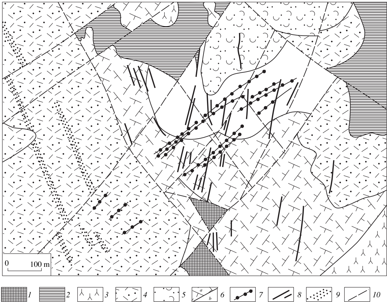
Fig. 2. Schematic geological setting of the Dukat silver deposit (Okhotsk–Kolyma watershed) [1]. (1) Triassic sandy–shaly sequences; (2) Lower Cretaceous terrigenous sequences; (3–5) Upper Cretaceous volcanogenic sequences: (3) andesite, (4) rhyolite, (5) felsite; (6) complex effusive–subvolcanic rocks: (a) stratified andesites, dacites, and rhyolites, (b) fluidal felsitic rhyolites; (7) basaltic andesite dikes; (8) ore bodies; (9) Sn-bearing chloritization zones; (10) faults.
