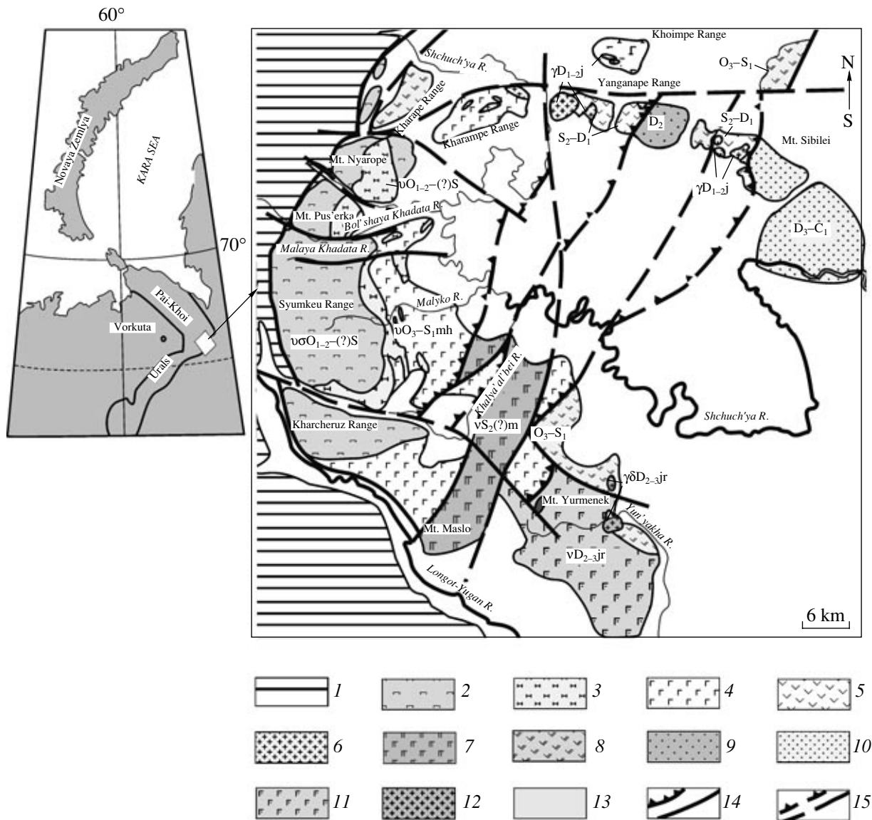
Fig. 1. Geological scheme of the Symykeu –Shchuch'ya area. Based on original data and materials reported by V.N. Okhotnikov, M.N. Kostyukhin, D.N. Remizov, A.K. Afanas'ev, V.N. Voronov, and S.N. Pchelintsev. Western Megazone: (1) Late Precambrian metamorphic sequences of the Nyarope–Kharbei zone; Eastern Megazone: (2–6) Symykeu subzone: (2, 3) Symykeu ultramafics–pyroxenite complex, (4) Malyko–Kharampe gabbroic and metagabbroic rock complex, (5) Yanganape volcanosedimentary sequence, (6) Yun'yakha gabbro–granodiorite–granite complex; Shchuch'ya subzone: (7) Maslo gabbroic complex, (8–10) volcanosedimentary and carbonate sequences, (11) Yurmenek biotite gabbro complex, (12) granodiorite and granite; (13) Mesozoic and Cenozoic sedimentary cover; (14, 15) faults.
