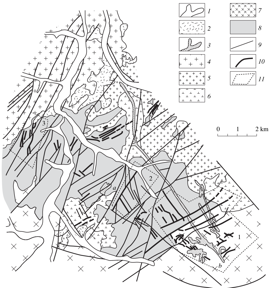
Fig. 1. Geological map of the Darasun ore group (based on materials of the Darasun geological-exploration expedition). (1) Alluvial sediments; (2, 3) Middle–Upper Jurassic Amudzhikan Complex: (2) volcanic rocks, (3) subvolcanic and dike porphyry rocks (diomite porphyries, granodiorite porphyries, granite porphyries, and others); (4) Triassic Amanan Complex (biotite–hornblende granites and granodiorites); (5, 6) Upper Paleozoic–Lower Mesozoic Olekma Complex: (5) biotite and leucocratic granites, (6) syenites, granosyenites, and quartz syenites; (7) Middle Paleozoic Krestov Complex (diorites, quartz diorites, and granodiorites); (8) Lower Paleozoic Kruchina Complex of metamorphosed gabbroic rocks (granitized gabbro, amphibolites, gabbro diorites, and troctolites); (9) tectonic fractures; (10) ore bodies; (11) deposits: (1) Darasun, (2) Teremkin, (3) Talatui. (a) Ring-shaped anomaly; (b) Darasun intrusion framework.
