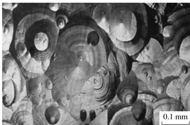
Fig. 4. Monocrystal of synthetic topaz grown on a seed parallel to {001} in acidic aqueous–fluoride fluids at 730°C and 150 MPa.
