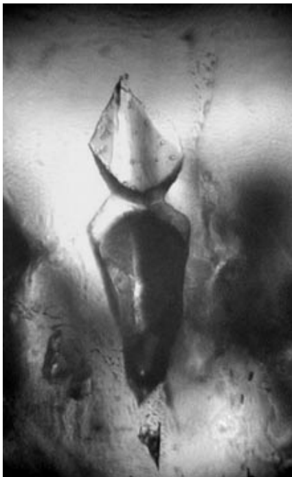
Fig. 8. Large three-phase fluid inclusion consisting of gas, liquid, and a solid phase (fluoride-silicate glass?) in synthetic topaz.
