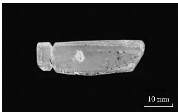
Fig. 4. Monocrystal of synthetic topaz grown on a seed parallel to {001} in acidic aqueous–fluoride fluids at 730°C and 150 MPa.
