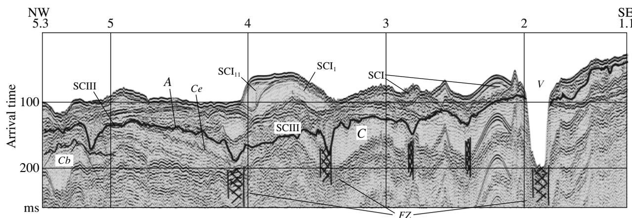
**Fig. 4.** A fragment of CSP section 200305\_01. (A) The base of Quaternary deposits; (Cb) the base of Vendian deposits; (Ce) erosional surface in Vendian deposits; (C) Vendian SC; (V) present-day incision; (FZ) fractured zones.
