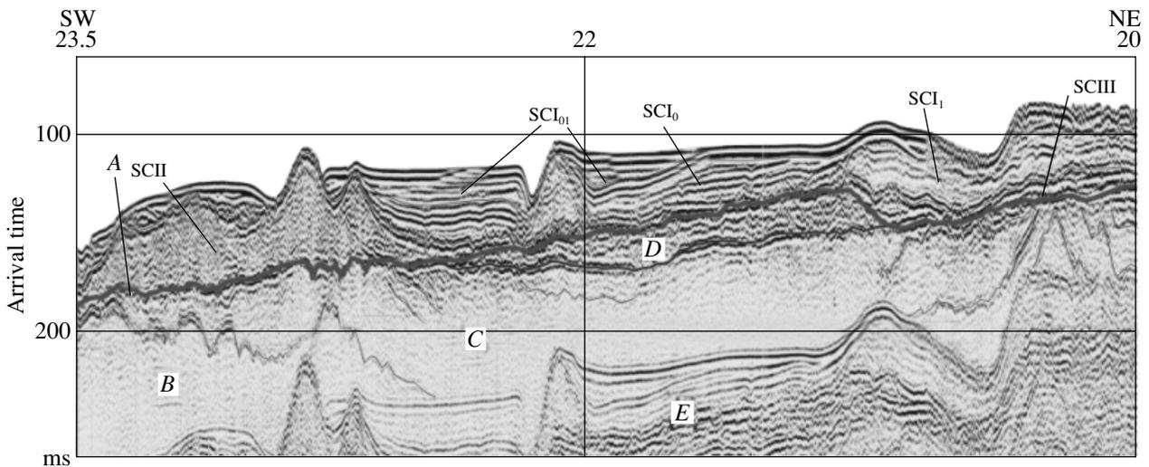
**Fig. 2.** A fragment of CSP time section 030305. (A) The base of Quaternary deposits; (B) Riphean SC; (C) Upper Riphean SC; (D) Vendian SC; (E) multiple wave.
