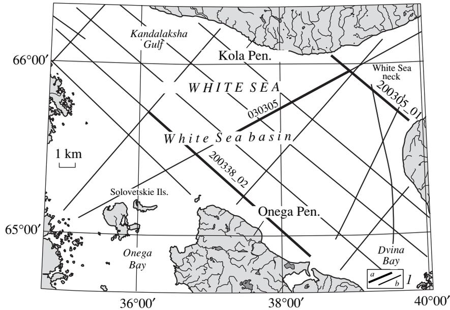
**Fig. 1.** Layout of seismoacoustic profiles in the White Sea. (I) Seismoacoustic profiles: (a) mentioned in the text, (b) others.
