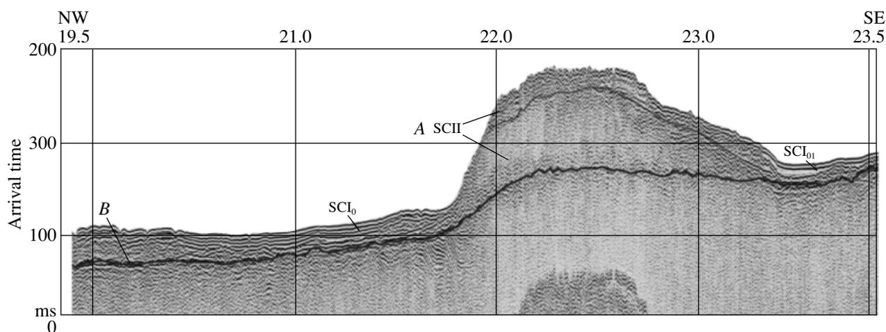
**Fig. 3.** A fragment of CSP section 200338\_02. (A) Glacial deposits of different ages; (B) the base of Quaternary deposits.
