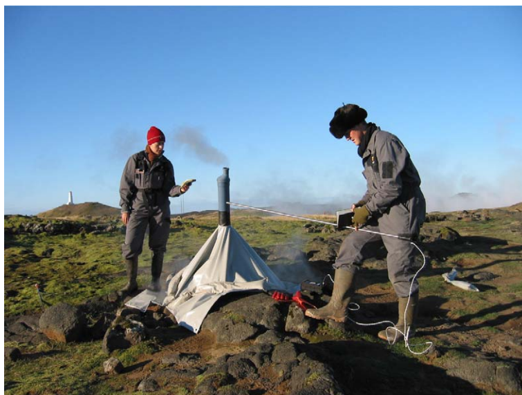
Fig. 2. Measurement of steam mass flow using hot-wire anemometer.
