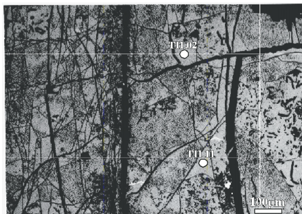
Fig. 1. Electron back-scattering image of a fragment of fossil tooth of a Cretaceous dinosaur, Allosaurid derived from the Hasandong Formation in the Gyeongsang basin, southeastern Korea. There are many cracks and voids indicated by dark color with low Z materials. Note that analyzed spots (TII.02 and TII.11) are located at relatively homogeneous regions.
