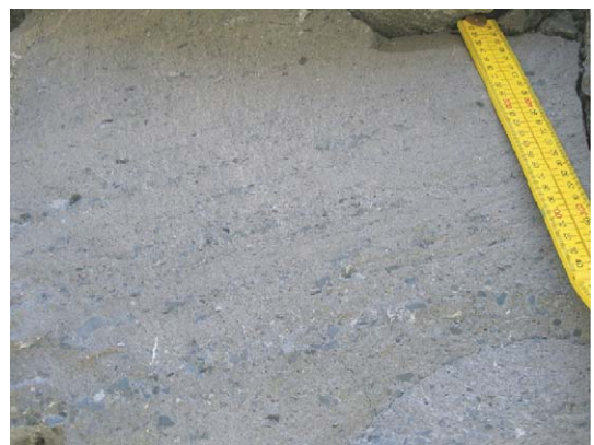
Fig. 5. Well-bedded volcanoclastic kimberlite (LVK) defined by the alternation of coarse and fine layers of lithic clasts. Locality is in the middle of the Jwaneng Central Pipe, Botswana.
