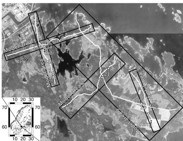
Figure 4. Reflection seismic profiles (white lines) and model areas (black frames). Refraction seismic profiles are shown with black and white dashed lines. Boreholes with recorded depth to bedrock are marked with white circles. On the aerial photo, the darkest areas are the sea or lakes, intermediate grays are forests, and lighter gray corresponds to wetland or agricultural areas.
