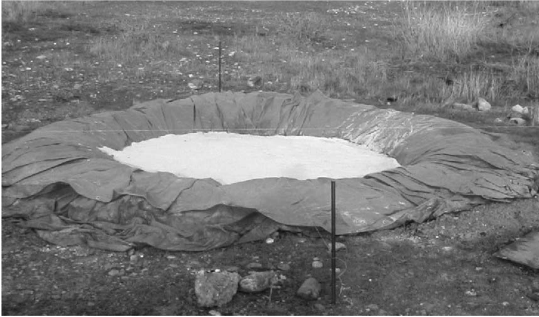
Fig. 1. The hemispherical test bed used in the experiments. It has been lined with a plastic sheet so that it can hold both sand and water. The sand surface is 2 m wide, and the depth below the sand surface is 1 m.
