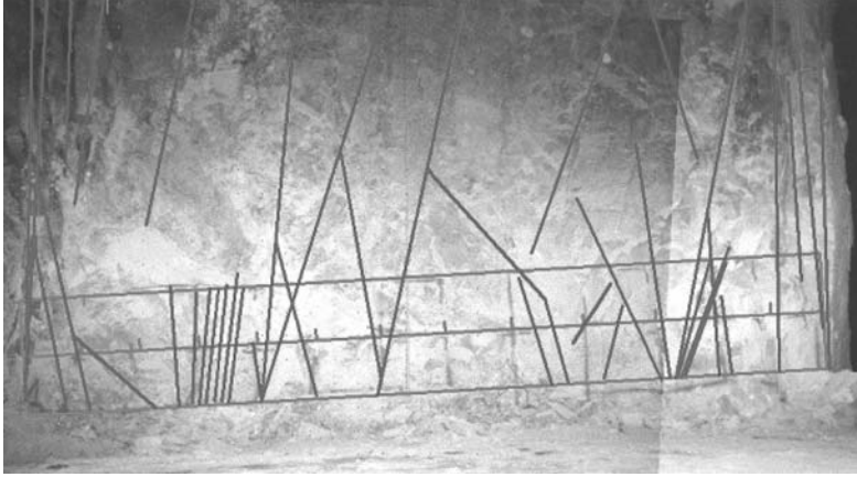
Fig. 6. Interpreted fractures on a mapped pillar face at Middleton Mine, facing NW. The pillar face (Face 1) is 13 \times 7 m. The 2 m high panel at the base of the pillar, where detailed mapping was undertaken, is also shown
