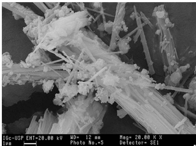
Fig. 2 SEM photograph of the natural zeolite with mordenite fibres ( \times 20,000 )
