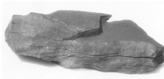
Fig. 2. The regime of F (Fushun oil shale) after primary migration simulation experiment.
